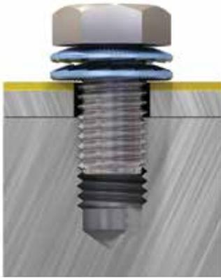
**1.** Put on the pre-assembled washer pair on the bolt and install the bolt in the threaded hole. Make sure the washers are oriented according to the picture.
